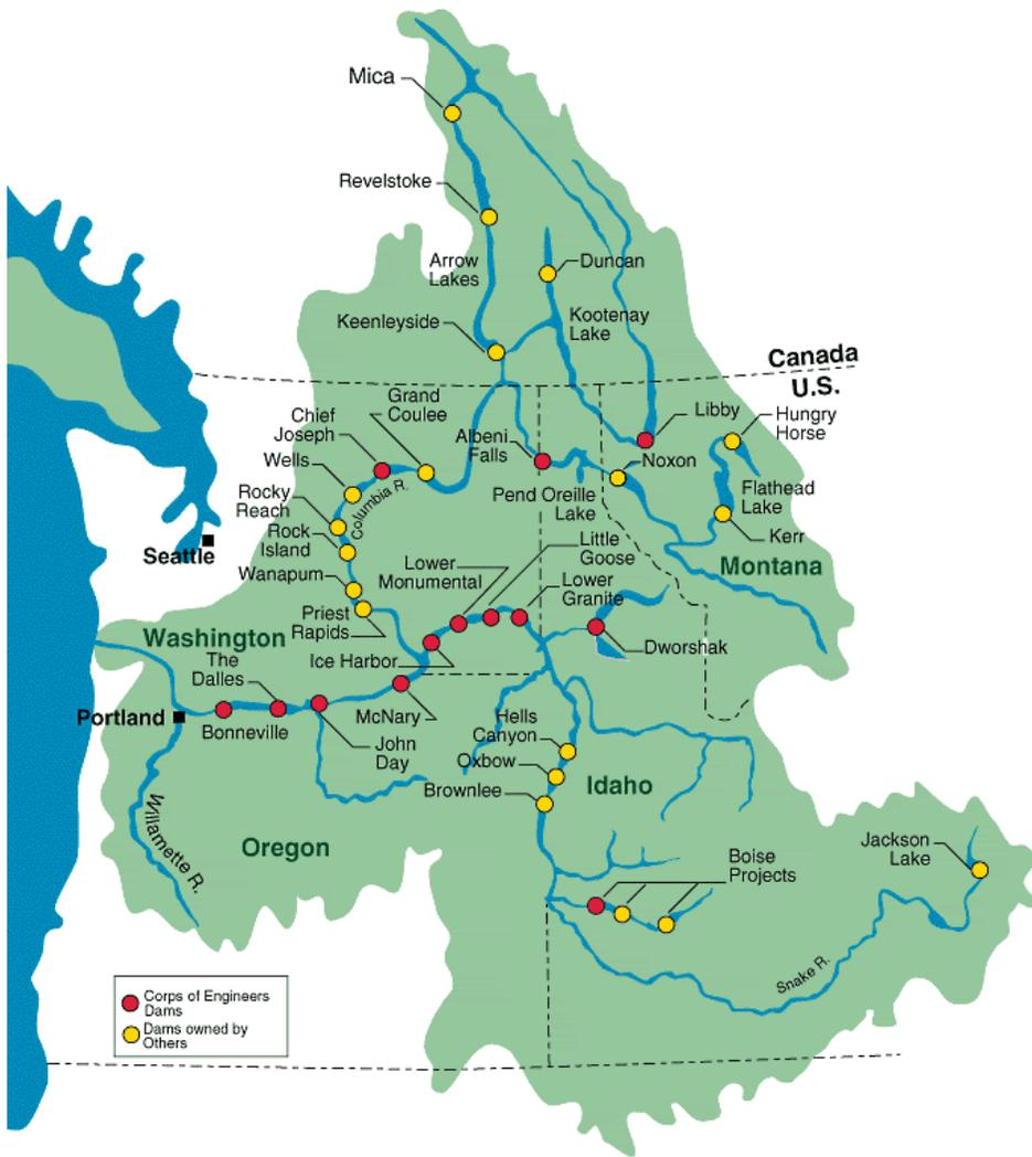
The Columbia-Snake River Basin. The four Lower Snake River dams are the four red dots in the center of the map, terminating just before the Idaho state line: Ice Harbor, Lower Monumental, Little Goose, and Lower Granite. Source: Courtesy of U.S. Army Corps of Engineers Northwest Division.
